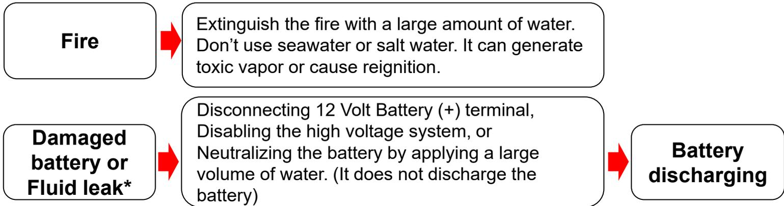
\*If electrolyte solution leakage, or any damage to the High-Voltage battery casing is observed.
